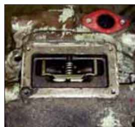
Asbestos isn't always obvious. Would you spot an asbestos gasket on an old engine, asbestos cement pipes or an asbestos-containing fuse-board? If you're not sure, the premises owner needs to get it checked out!
